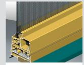
Custom sub-sill (flashing tray) standard on 466 windows. This sill detail shows our custom concealed electric winder box. Winder box recessed to accept flyscreen as shown above.
